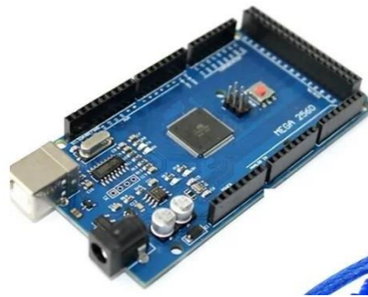
Figure 5: This is the Arduino Mega, which contains the microcontroller.
