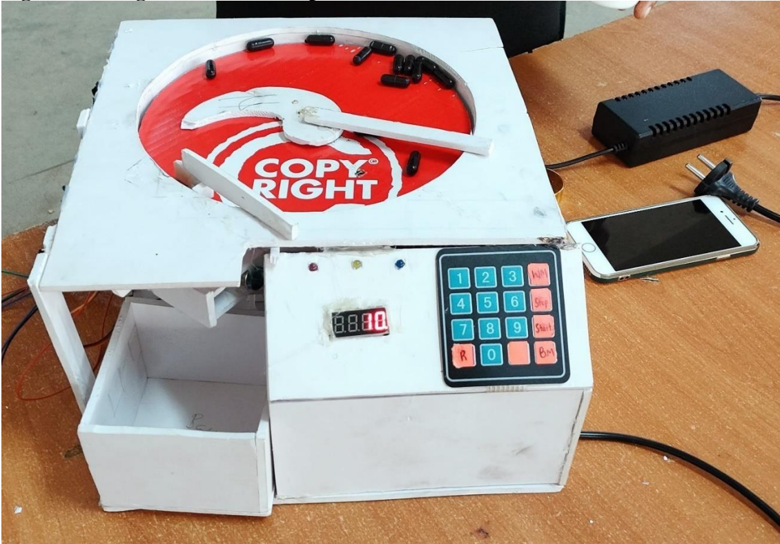
Figure 18: The Automated Tablet or Capsule Counter Device
