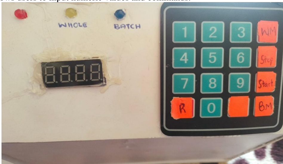
Figure 17: Keypad and the LEDs indicating whole mode and batch mode of counting
